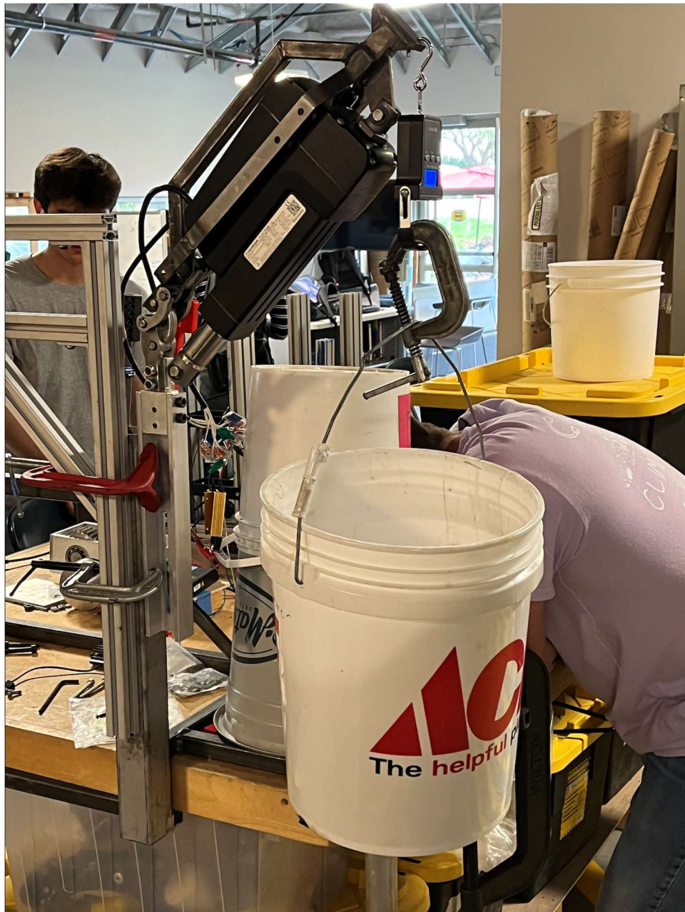
Figure 28. Load carrying capacity test setup.
