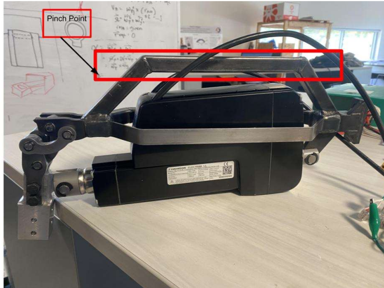
Figure 22. Pinch point between the linear actuator and frame.
