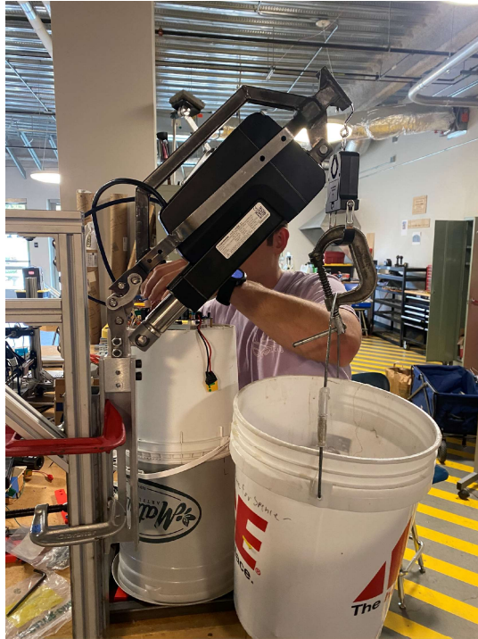
Figure 19. Experimental apparatus/setup for load capacity and noise tests.
