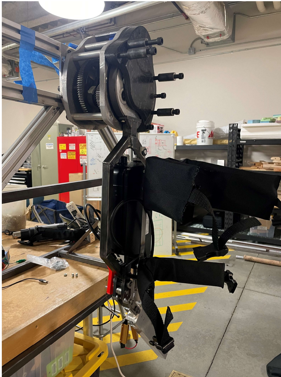
Figure 20. Knee joint integration with hip joint and tibia structure.
